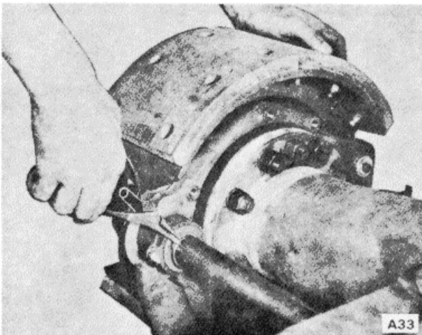
Figure 9C-20. Installing Camshaft Retaining Ring
