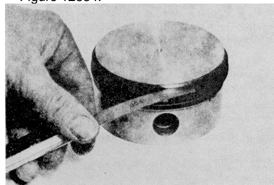
Figure 12B-34. Check Ring Groove Wear
