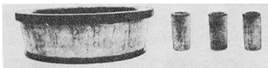
Figure 9D-13. Pitted Bearings
