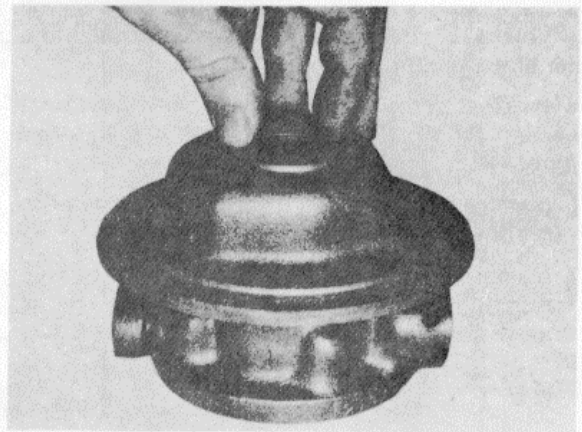
Figure 16L-25. Installing the Bearing Washer (Turbine End)
