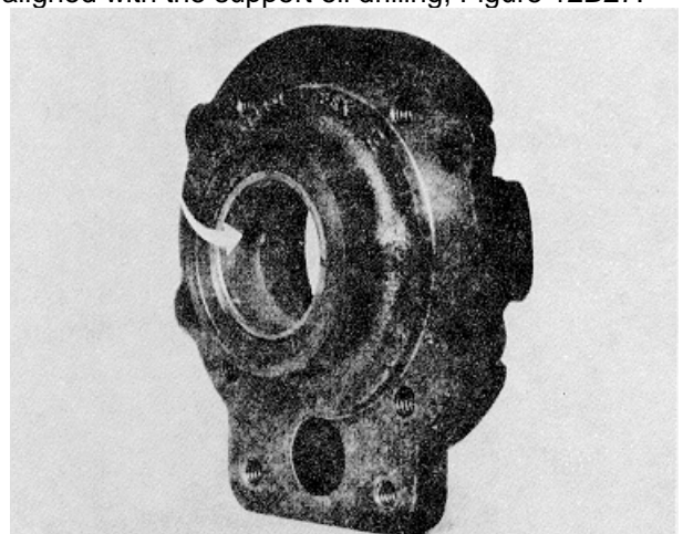
Figure 12B-27. Align Bushing Oil Hole
